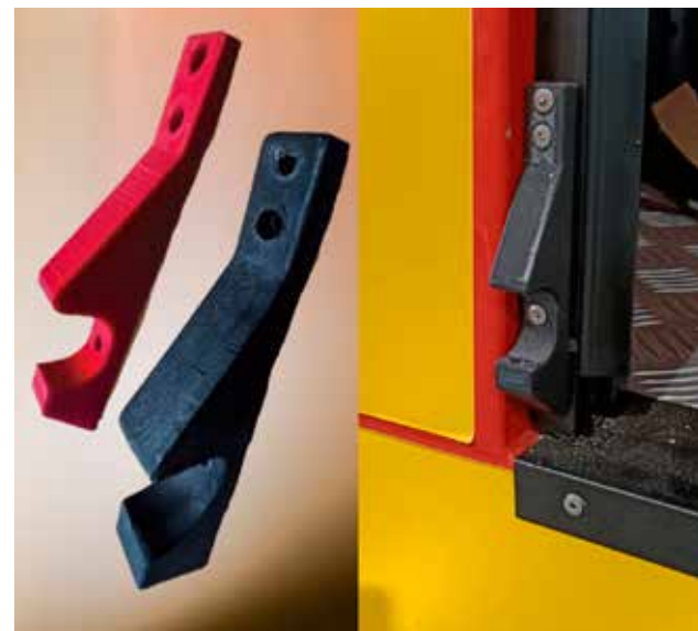
This Fire Truck Boot Loader, 3D printed at UNGSC, enabled an inactive asset valued at over 300K to once again become operational. Image courtesy of UNGSC.
